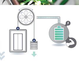
Stores the energy wasted by the elevator when motor brakes to return it in the next consumption trip. Energy savings up to 70% with no harmonic distortion and no added stand-by consumption with a simple two-wire con-
